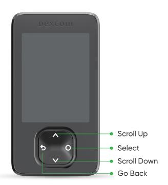
To turn the receiver on press and hold the **Select** button for 3-5 seconds. The receiver walks you through setup step-by-step.
